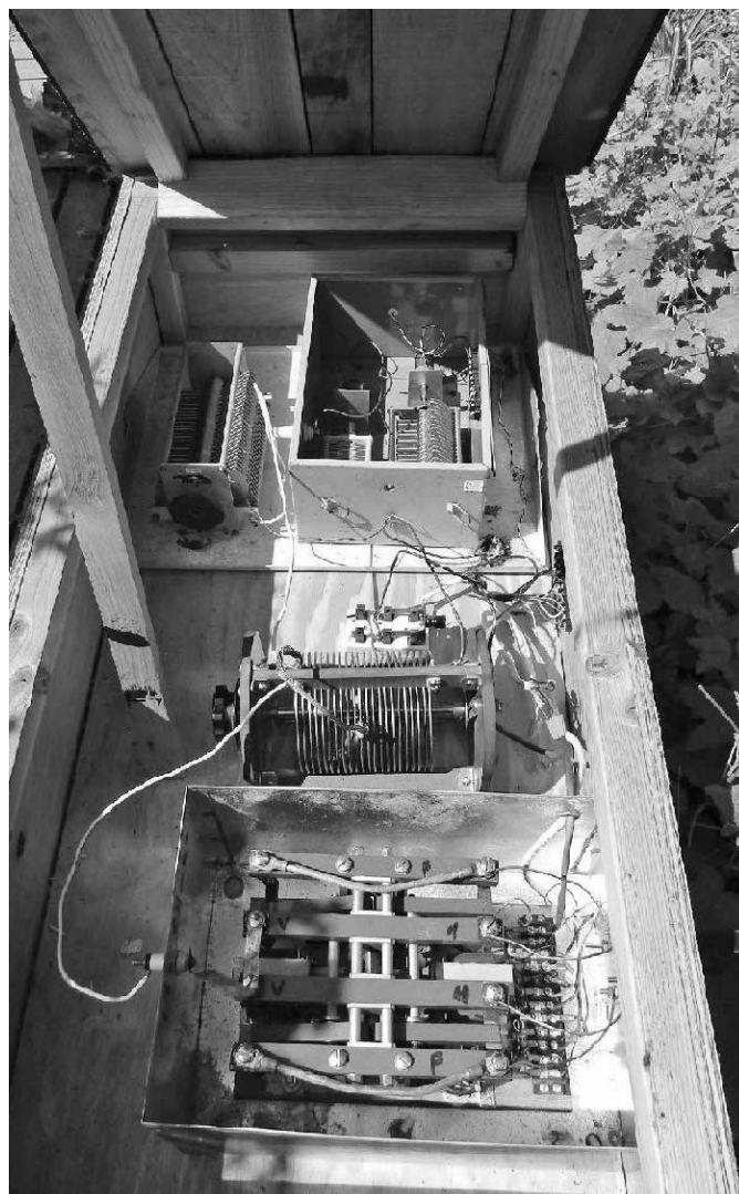
Photo B — This photo is a view of the tuning networks inside the tuning box from Photo A. Near the bottom of the photo you can see my heavy duty antenna transfer switch. This was surplus from a high power AM broadcast facility. Vacuum switches or high voltage ceramic switches can also be used.
